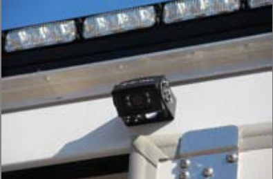
Reverse cameras are standard, and are mounted to assist the driver in positioning over the manhole.
