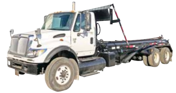
2006 International 7600 w/ Cascon/Wastequip Endless Chain Hoist
