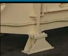
Raiser kit allows for easy cleaning and clearing around baler.
