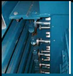
Maren's unique 100% gear driven twister maintains timing and avoids problems common with chain driven systems.
