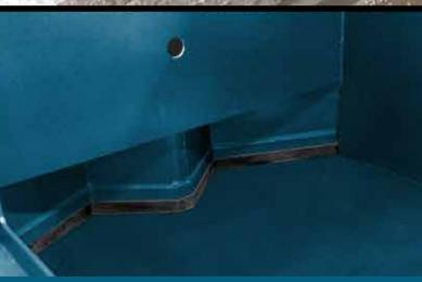
Hardened tool steel progressive shear blade and 30" penetration all but eliminates shear jams.
