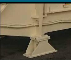
Raiser kit allows for easy cleaning and clearing around baler.
