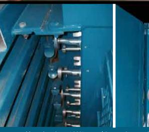
Maren's unique 100% gear driven twister maintains timing and avoids problems common with chain driven systems.
