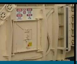
Lower ram chassis inspection door for easy maintenance access.
