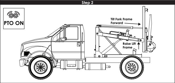
2. Engage the PTO and raise the lift frame high enough to clear the truck frame. Tilt the fork frame forward.
