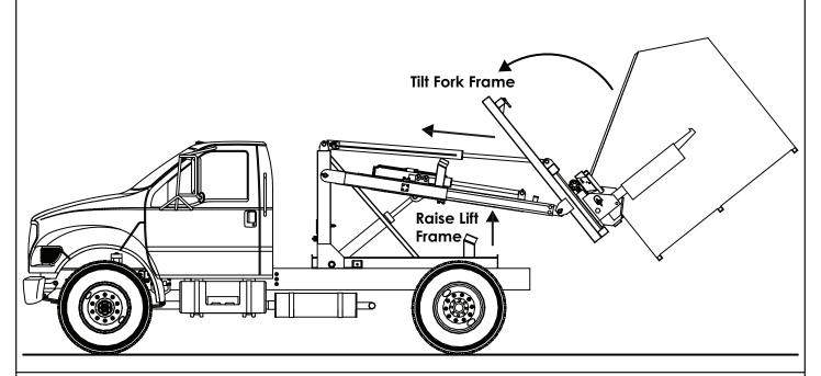
5. Raise the lift frame and tilt the forks up high enough to clear the truck frame.
