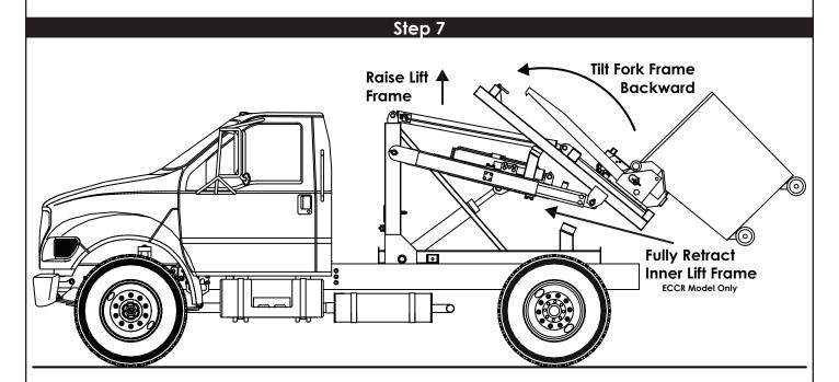
7. Raise the lift frame high enough to clear the truck frame. Fully retract the inner lift frame (ECCR Model Only). Tilt the fork frame all the way up so full contact is made with the rest pads.
