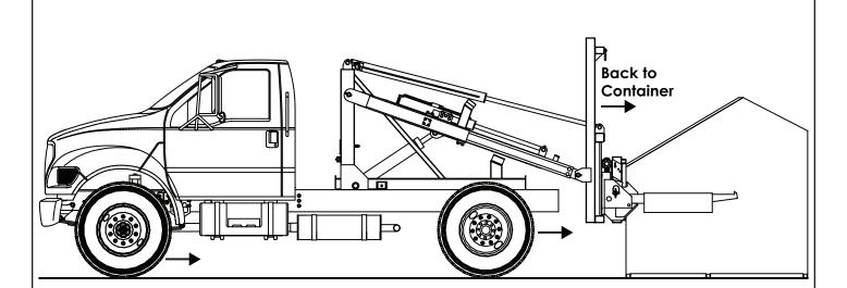
4. Slowly back the truck up to the container. Continue backing until the forks extend through the pockets and the container contacts the bumpers on the fork frame.
