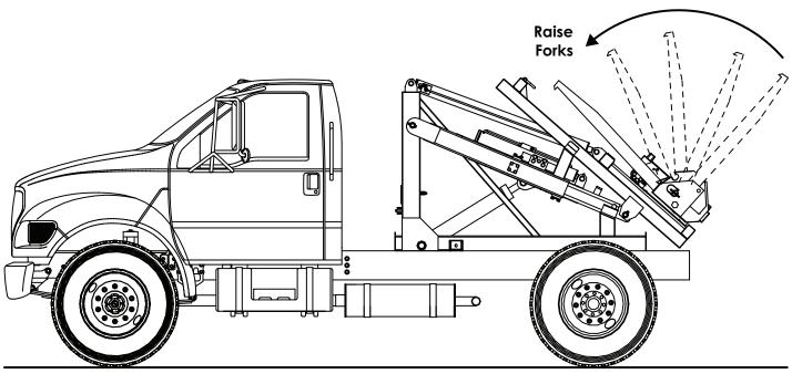
1. If the forks are in the extended position, manually rotate them to the stored position. Lock the forks in place with the fork stop pins.
