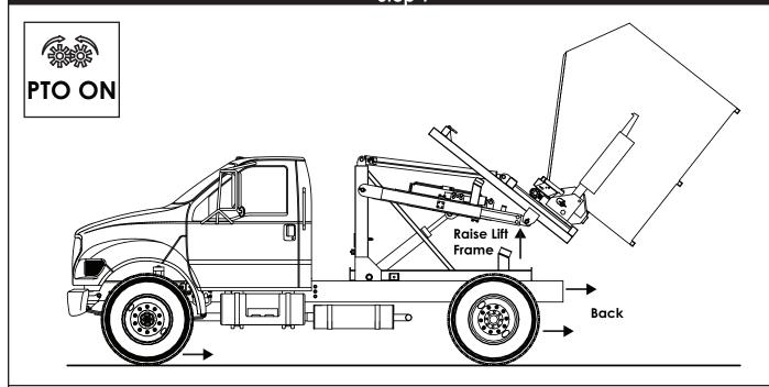
1. Back the truck up close to where the container will be placed. Engage the PTO and raise the lift frame high enough to clear the truck frame before tilting the fork frame.
