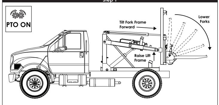
1. If the forks are in the stored position, engage the PTO and raise the lift frame high enough to clear the truck frame. Tilt the fork frame forward to allow easy manual rotation to the down position. Lock the forks into place with the fork stop pins.
