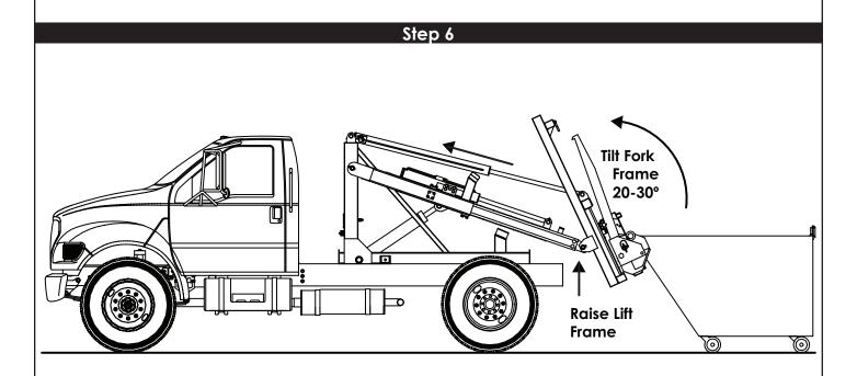
6. Raise the lift frame until the trunnion bars are securely located in the slots. Tilt the fork frame up approximately 20 to 30 degrees. Put both trunnion bar stops in the 'locked' position (See next page).
