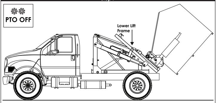
7. Lower the lift frame completely and disengage the PTO. Note: Check local DOT lighting regulations before transporting.
