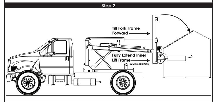
2. Tilt the fork frame forward until the container is parallel with the ground. Fully extend the inner lift frame (ECCR Model Only).
