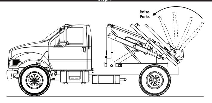
1. If the forks are in the extended position, manually rotate them to the stored position. Lock the forks into place with the fork stop pins.
