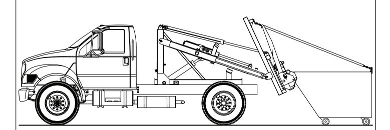
7. Attach a chain from the top of the fork frame to the container. Run the chain through a pipe to prevent the container from tipping forward if the truck has to make a sudden stop.
