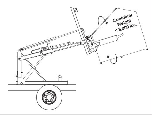
**AWARNING** Failure to tilt forks up before rotating container may result in container sliding off of forks with possible damage to equipment and injury to personnel
