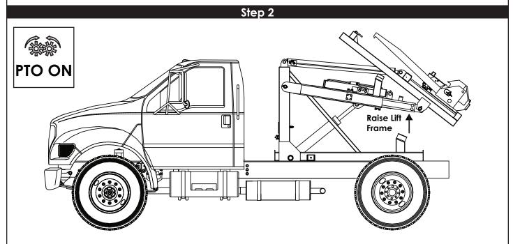
2. Engage the PTO and raise the lift frame high enough to clear the truck frame.
