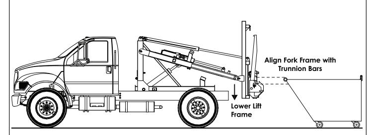
4. Align the fork frame with the trunnion bar on the container by lowering the lift frame and tilting the fork frame.
