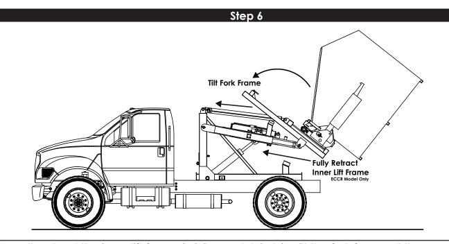
6. Fully retract the inner lift frame (ECCR Model Only). Tilt the fork frame all the way up so that full contact is made with the rest pads.
