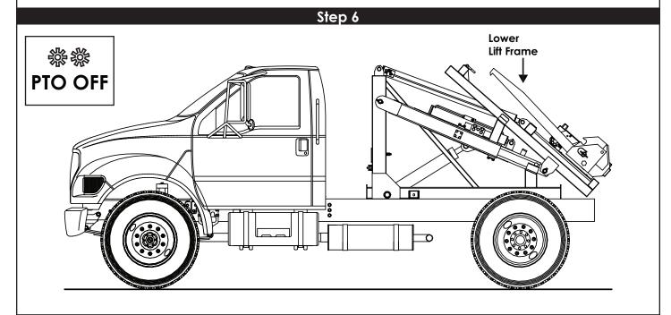
6. Lower the lift frame completely and disengage the PTO.
