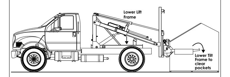
3. Lower the lift frame until the container is fully rested on the ground. Tilt the forks down enough to clear the container pockets.
