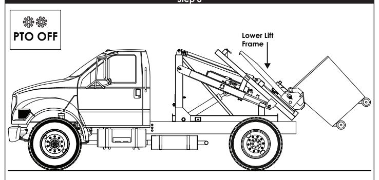
8. Lower the lift frame completely and disengage the PTO. Note: Check local DOT lighting regulations before transporting.
