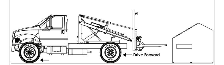
4. Slowly pull the truck forward until the forks are completely clear of the container pockets.
