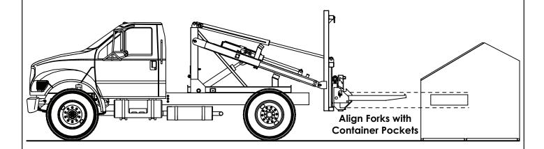
3. Align the forks with the container pockets by lowering the lift frame and tilting the fork frame.
