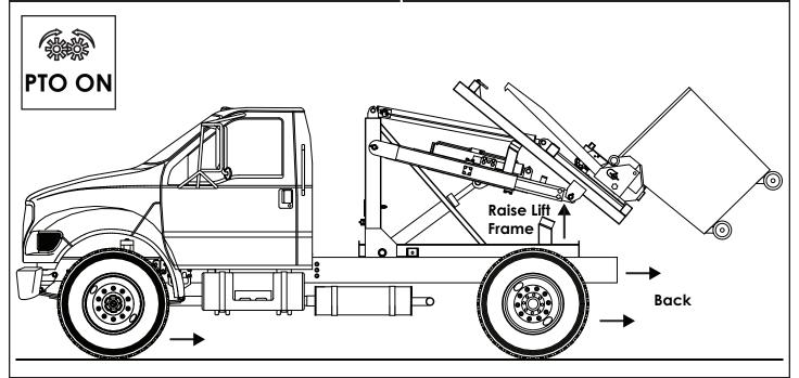
1. Back the truck up close to where the container will be placed. Engage the PTO and raise the lift frame high enough to clear the truck frame.
