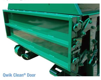
The **Qwik Clean** door on the packer end makes cleaning out behind the ram in cylinder area a snap. The door has miniature hinges, a door seal, and a ratchet binder.
