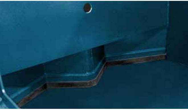
Hardened tool steel progressive shear blade and 30" penetration all but eliminates shear jams.
