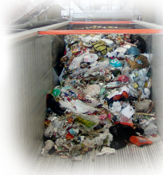
The BlokPak 3000 forms 10' (3m) logs of densely packed waste.
