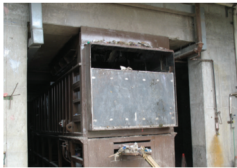
This M-1475XW Transfer Station Compactor is fed via a tipping-floor and features the Scissor trailer connection system.
