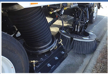
VACUUM AND BRUSH REMOVAL OF DEBRIS
