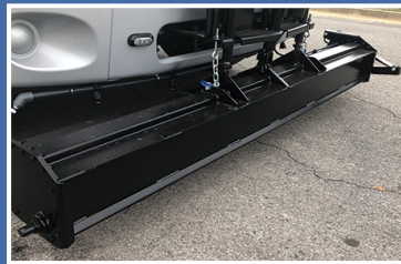
POWERFUL MAGNET TO COLLECT FERROUS MATERIAL
