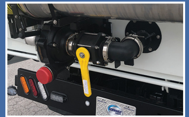
GLYCOL RECOVERY FOR PICKING UP DE-ICING FLUID
