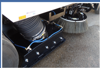
VACUUM AND BRUSH REMOVAL OF DEBRIS
