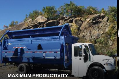
The Top Select is equipped with dual hydraulic cylinders featuring adjustable cushions for seamless operation of the loading bucket.
