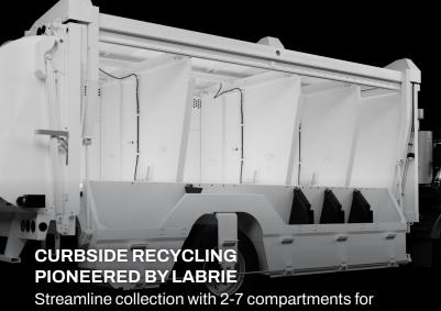
Streamline collection with 2-7 compartments for precise sorting. Unique over-the-top dumping. Add optional cart attachments for easy roll cart pick-up.
